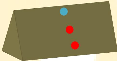
Figure 2: Here is shown 3 different points of the temperature test. Blue colour: two tests done every day (one test 0cm and another test at 50cm depth). Red colour: tests done at 0cm, 50cm and 100cm depth.
