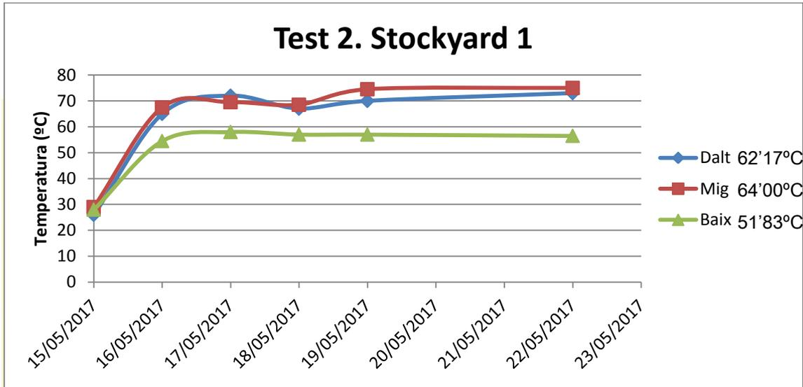
Graphic 3: Temperature curve from Stockyard 1. Test 2
